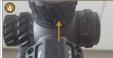
REINSTALL AT "6" (-1.0 MRAD)
